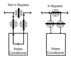
Figure 5 Typical Globe Valve Bypass System
